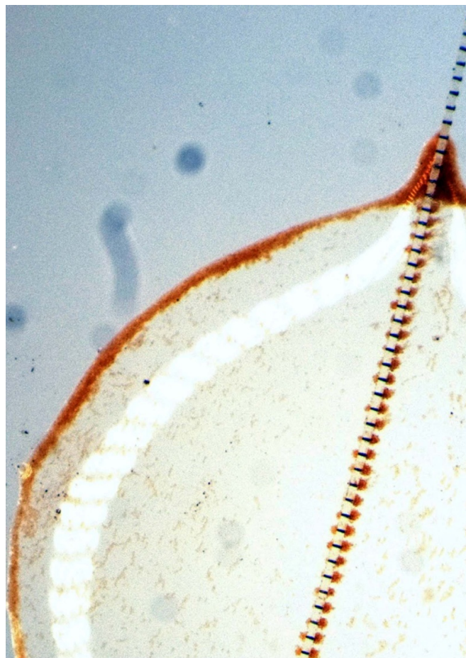
Figure 18. Collective transport of magnetic microparticles on an artificial microtubule near a droplet.
