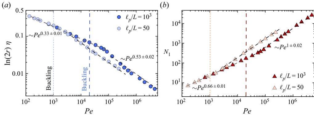
Figure 3. (a) Polymer viscosity  $\eta$ , and (b) normal stress difference  $N_1$  as functions of  $Pe$  for  $(\ell_p/L, r) = (1000, 220)$  and  $(50, 100)$  in 2-D simulations. Vertical dashed lines show the two buckling thresholds, which correspond to the same value of  $\bar{\mu} = \bar{\mu}^{(1)}$ .
