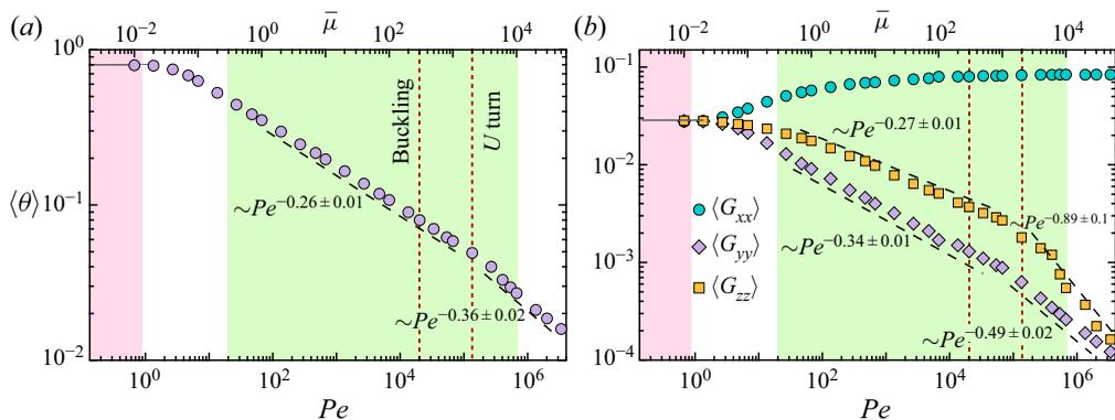
Figure 2. (a) Mean polymer orientation  $\langle \theta \rangle$ , defined as the angle made by the dominant eigenvector of the gyration tensor with the flow direction, as a function of  $Pe$  and  $\bar{\mu}$ . (b) Diagonal components  $\langle G_{xx} \rangle$ ,  $\langle G_{yy} \rangle$  and  $\langle G_{zz} \rangle$  of the mean gyration tensor.
